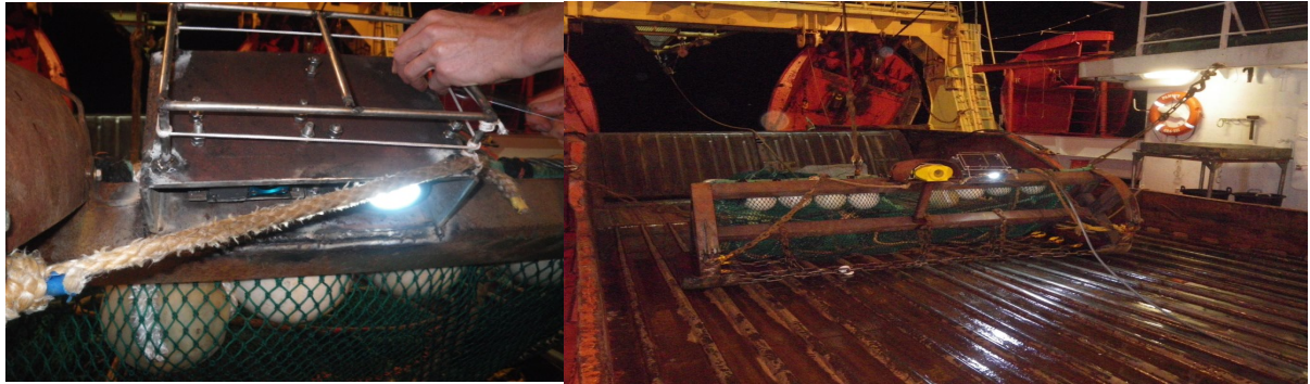
Figure 2. Framework and housing for GoPro camera (left), and fitted to the beam trawl (right)
