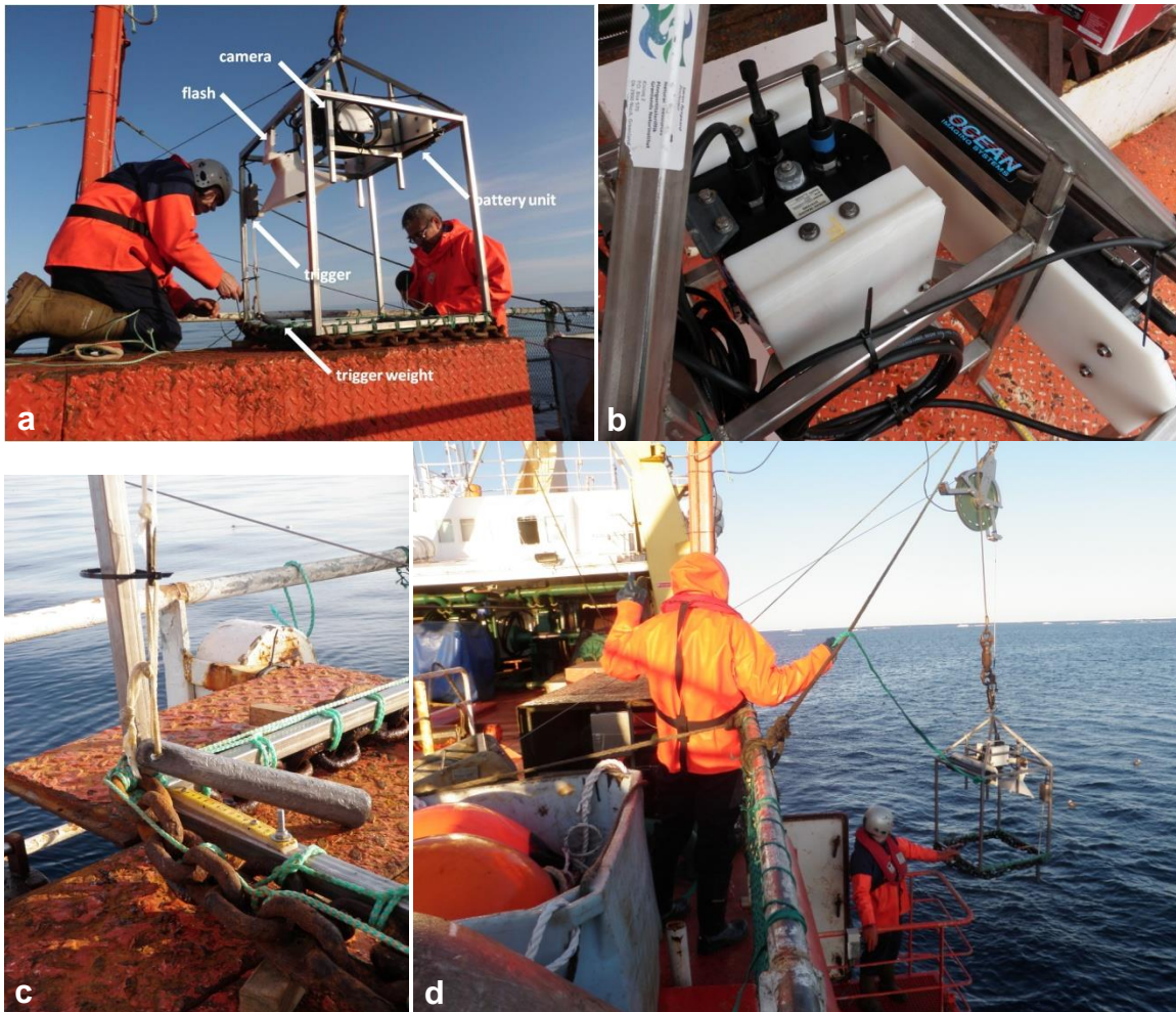
Figure 2. (a) The apparatus consisted of a downward facing stills camera, flash unit, battery pack, trigger and trigger weight. (b) Detail of camera unit and connectors. (c) The trigger weight was adjusted to hang ~8cm below the frame. (d) The apparatus was deployed and recovered using the starboard winch wire.
