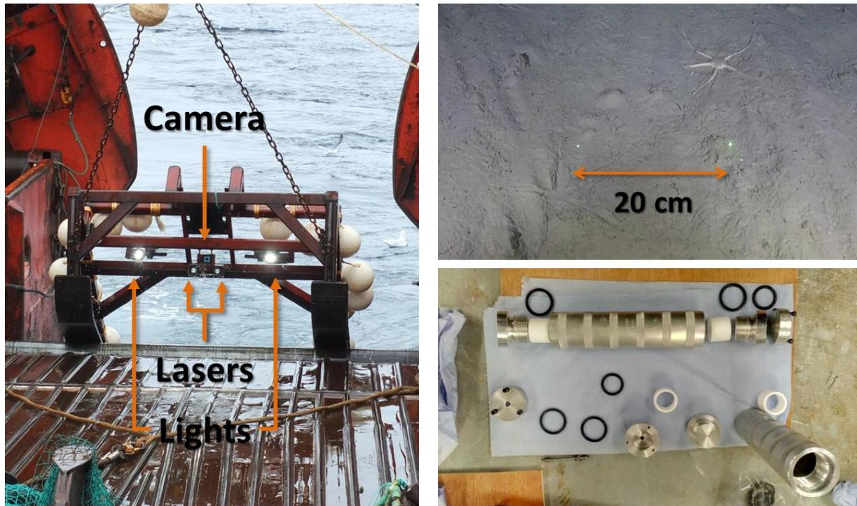
Figure 2: Clockwise from left, camera sled showing camera lights and laser positions, example still from video showing laser dots 20cm apart, purpose built laser housing.
