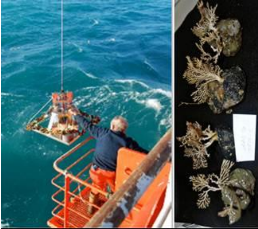
Figure 2. Grab sampler in action and example specimens
